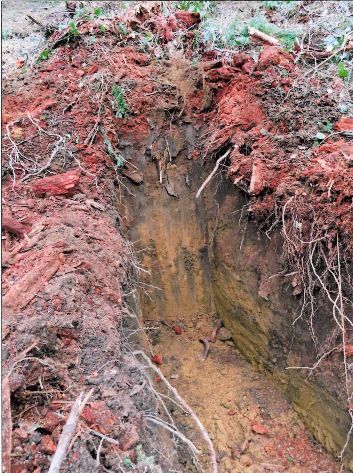
Figure 6: Test Pit 2 with brown clay-silt to 5 ft deep, capped by a layer of organic topsoil and mixed silt. This is decomposed mudstone from chemical weathering. No colluvial textures; Stiff Consistency.
